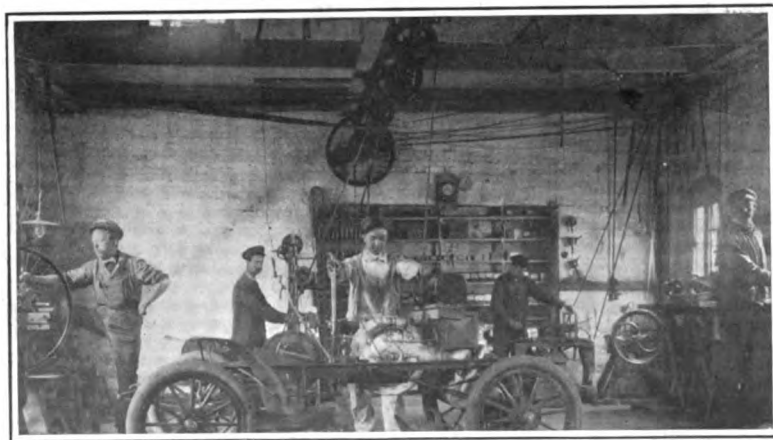
RUNNING MACHINERY IN A GARAGE TEMPORARILY WITH AN AUTOMOBILE.
